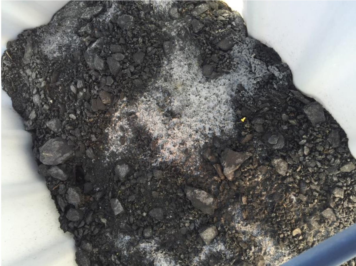
Figure 7: Alum shale surface inside a pallet experiment, most likely AT3K or AT4K due to the lime residues. The material is visibly heterogeneous in terms of grainsize.
